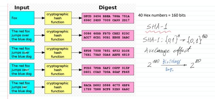
A cryptographic hash function (specifically <u>SHA-1</u>) at work. A small change in the input (in the word "over") drastically changes the output (digest). This is the so-called avalanche effect.
